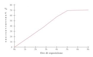
The present graph show the lubrificant substance concentration at different time of exposition of GLISS\* F at the constant temperature of 65 °C
