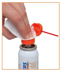
For improved wet-dry cleaning, use the Sticklers™ Fiber Optic Splice & Connector Cleaner (#MCC-POC03M) which comes in a pocket-size spray canister. This cleaning fluid is strong, nonhazardous and dries fast.
