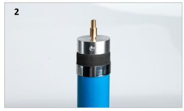
Screw the 8-32 end of the thread adaptor into the hold on the top of the platform located on the <u>Telescoping Pole RDT-18K)</u>.
