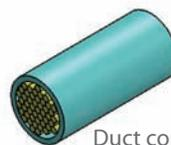
Duct containing 48 x Ø 1.2mm cable
