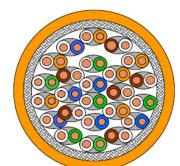
Special Note: The conductor diameter is smaller compared to the standard cables. This leads to an increased attenuation and therefore the operating distance is reduced (80 m instead of 90 m installation cable in standard permanent link).
