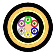
• Central Strength Member (CSM): glass fibre reinforced plastic rod (FRP).
