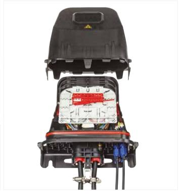
The Fibre Closure BPEO size 0 is equipped with different sized cable entry ports to accommodate different cables sizes. The description of the cable entry kit indicates the diameter of the cables that can be accommodated within each external cable assembly module (ECAM) and within the closure port in the base.
