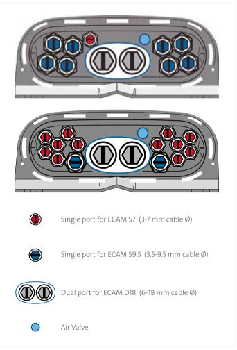
One dual port for double ECAM D18, two single ports S9.5, and 12 single ports for ECAM S7
