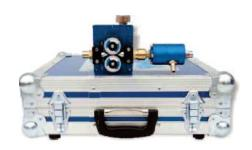
BDJ BUDGET/ BDJ BUDGET PLUS micro cable blowing machine is dedicated for last mile of FTTH network. Depending on the quality of the laid micro duct route and cable stiffness, BDJ Budget/Budget Plus can be used to blow cable sections up to 700m. Very easy to use. BDJ BUDGET is powered by a cordless drill/drive. BDJ Budget Plus model is equipped with an openable blowing head, so you can access your cable and remove it from the microduct easily, without cutting it.
