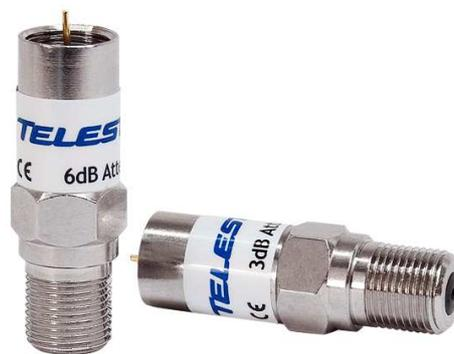
Inline return attenuators are used when extra attenuation is needed only the return path. The forward path will only be attenuated by < 1.0 dB. With F-female / F-male connectors, the attenuators can be mounted directly on an F-connector without the need of adapters. The return attenuators can be used for example to reduce ingress problems.
