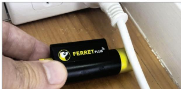
3. Using the NCVD function with the Ferret Plus camera in your hand will have the greatest sensitivity for voltage between 90V AC and 600V AC.
