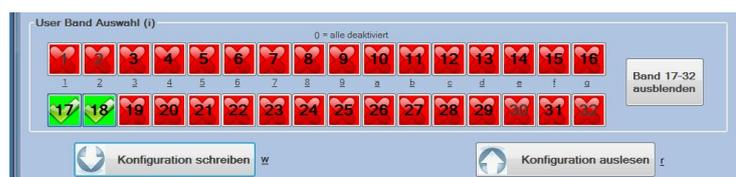
Depending on the application, more than one User Band ID per antenna wall outlet may be released. For example, two User Band IDs are required for twin receivers.
