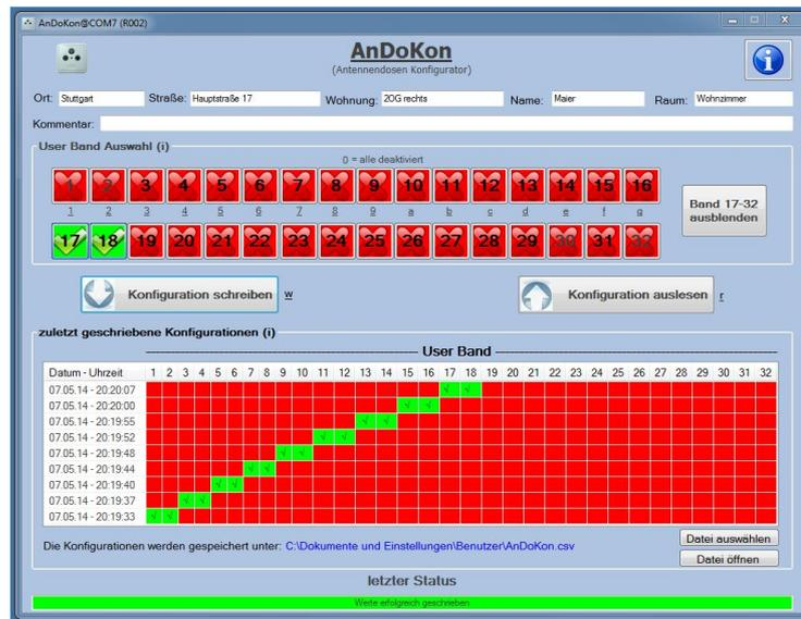
With the AnDoKon software, the antenna wall outlets of type SSD 6-xx can be read out "Konfiguration schreiben" as well as programmed "Konfiguration auslesen".
