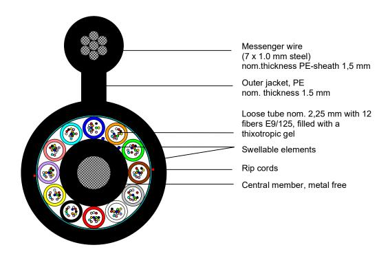
Principle drawing: example A-DQT2Y 12x12 E9/125 0,36F3,5 + 0,22H18 LG (7x1,0mm)
