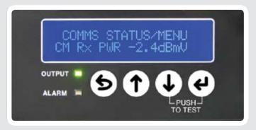
Displays Transmit (TX) and Receive (RX) power levels (dBmV) to ensure communications with the network operating center
