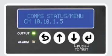
Displays IP address to verify network communication
