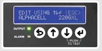
Battery set-up menu allows the selection of AlphaCell models to optimize charging and prolong battery life
