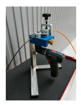
BUDGET EASY SET is a set of products including BDJ BUDGET or BUDGET PLUS unit. BDJ BUDGET micro cable blower is dedicated for the last mile of FTTH network. The obtainable blowing lenght is 500-700 m. EASY SET product box includes: BUDGET or BUDGET PLUS cable blowing unit, fully integrated drill/drive and a stainless steel mini-tripod. Easy to operate and ready to work solution.
