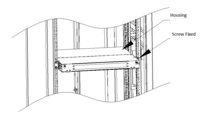
Figure-1. Frame Installation
