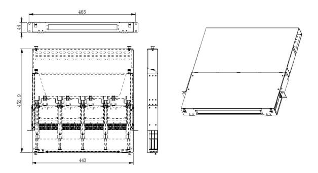
144-core MPO Pre-terminated Rack mount(Metal material)
