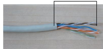
Strip approximately 30mm of the cable jacket, and separate to 4 pair each.
