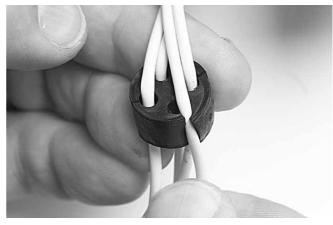
5.4.1 Insert the pigtails or jumpers in the rubber wrap around seal of the pigtail seal.
