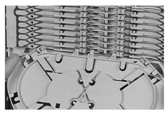
3.4.1 Install the splicing tray by pushing the lip on the groove plate slightly up with the tray and move the tray lateral from left to right into the hinging cavity.
