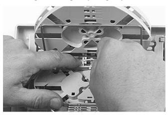
5.3.1 Guide the fibers to the cassette through the groove under the tray hinge.
