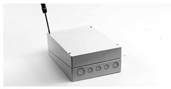
3.1.1 Unlock the screws and remove the cover.
