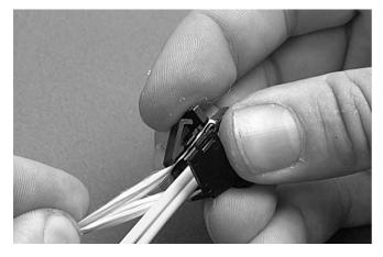
5.2.7 Close the KTU connector by snapping the lid, and pull on the Kevlar to slide the inner part backwards as far as possible.
