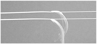
5.2.4 Remove the pigtail jacket up to the mark. Cut away the Kevlar up to 50mm-100mm from the ring cut.
