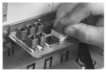
5.1.1 Connector adapters have to be installed in the patch panel.Push the adapter from the top in the patch panel and slide it in position.
