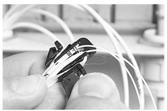
5.2.6 Take the two pigtails and bend the Kevlar over the inner part lips back between the two parts of the KTU.Mark the pigtails 50 mm away from the connector.
