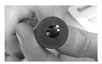
4.1.2. In case the cable diameter does not match with the diameter of the gland seal, remove the plastic nut, metal ring and rubber seal inside the gland and peel out some of the break out rubber rings up to the right diameter.
