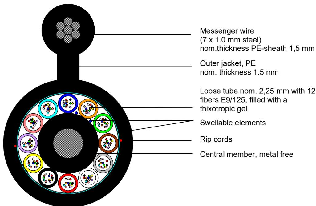
**Principle drawing:** example A-DQT2Y 12x12 E9/125 0,36F3,5 + 0,22H18 LG (7x1,0mm)
