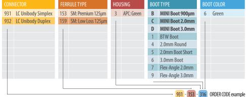
**Note:** Other ferrule ID size are available SM 126μm SM 125.5μm MM 230μm MM 144μm
